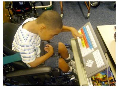
n cases where a person does not have reliable muscle ontrol in the hands for precision movements, an daptive keyboard can be useful.
