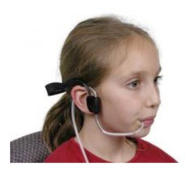
Similar in functionality to the single switch, sip and puff switches are able to interpret the user's breath actions as on/off signals, and can be used for a variety of purposes, from controlling a wheelchair to navigating a computer.
